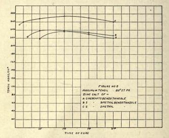
formula. The results are shown in Tables IIIa and IIIb and the tensile-time curves in Figs. 3 and 4.
