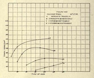
compounds resembles 1-mercaptobenzothiazole in certain parts of its structure. The results of these tests are recorded in Table IV and shown graphically in Fig. 5.
