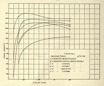
taken into consideration. The results of such tests are given for each cure in the tables in the column "State of Cure." In some cases the cures were not sufficiently close so that, for example, a 5-minute cure might be judged by means of these tests to be undercured, while a 10-minute cure would be considerably overcured. In such cases the writers have interpolated for the time of best technical cure.
