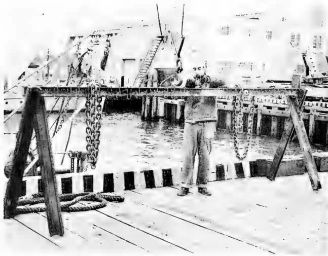
FIGURE 3. BIOLOGICAL FOULING RACK AS ORIGINALLY CONSTRUCTED
