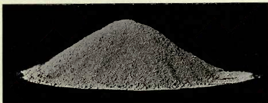
Acid Phosphate, Actual Size, as Cut Out of Den 15 Minutes after the Last Mix was Dumped into Den Note its granular form and absence of lumps---95 per cent passed a 6-mesh screen
