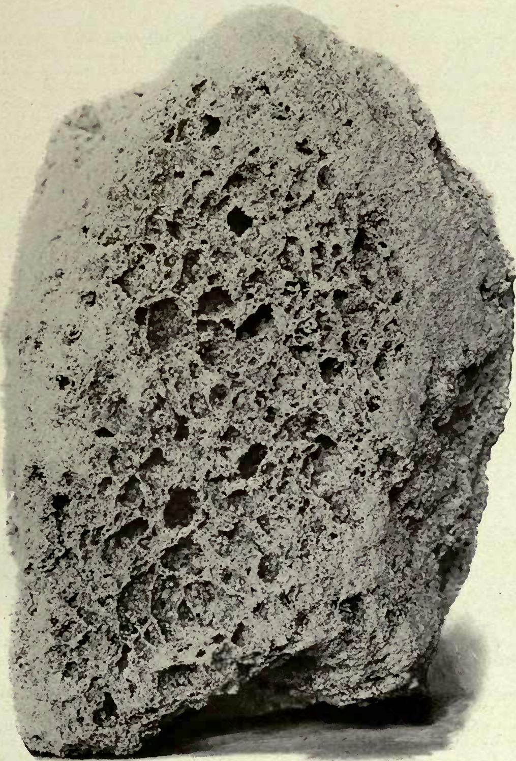
Photograph of Acid Phosphate Removed from Sturtevant Den after Fifteen Minutes set (Three times actual size)
