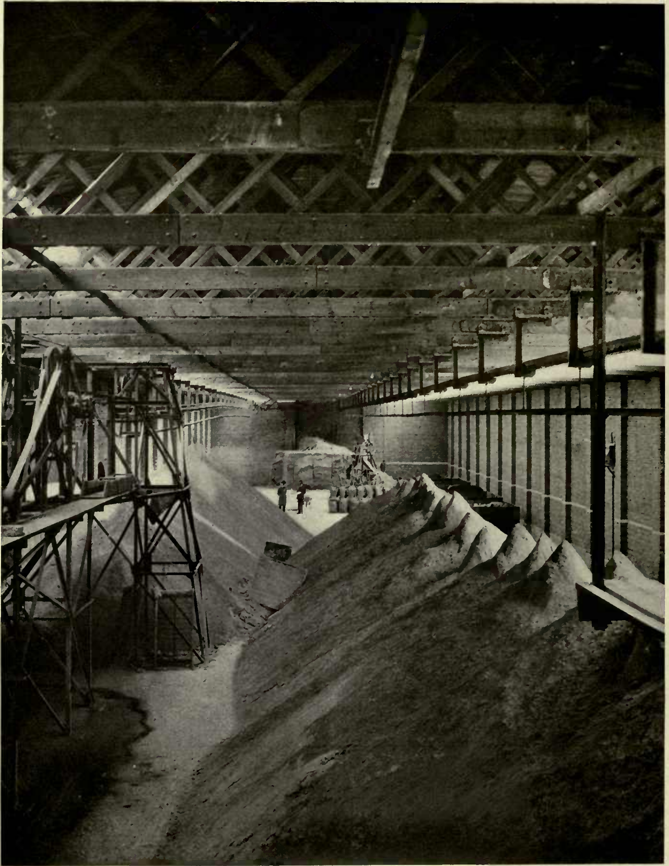
Acid Phosphate made by the Sturtevant Process being bagged and shipped without milling or screening Note absence of lumps (see page 26)
