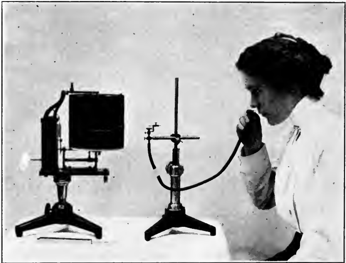
FIG. 86. — Recording the nasal current and vibrations.
