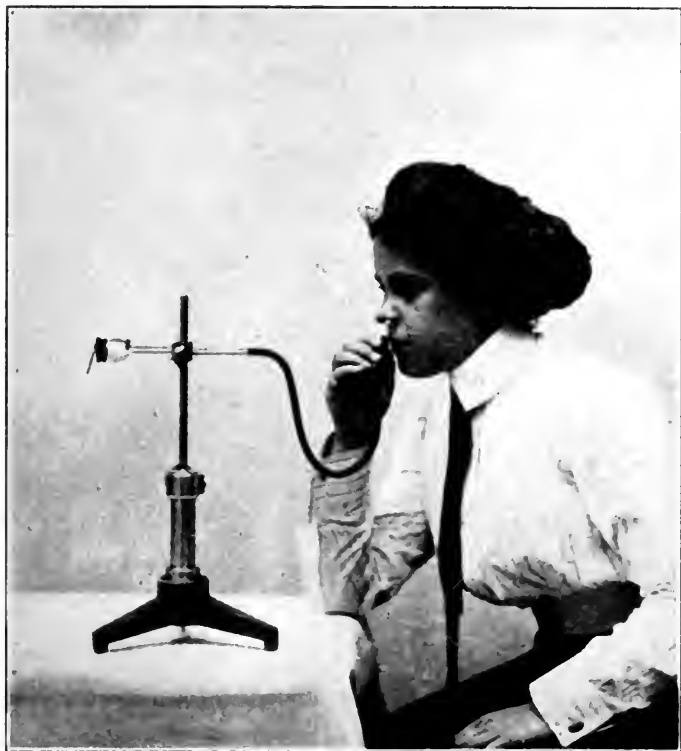
FIG. 43. — Tambour indicator used for the nose.
