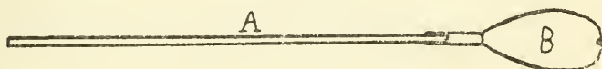
FIG. 14.—A lance bomb. The wooden handle A enables the charge B (7 lb. of high explosive) to be whirled round the head and hurled a distance of about twenty yards.
