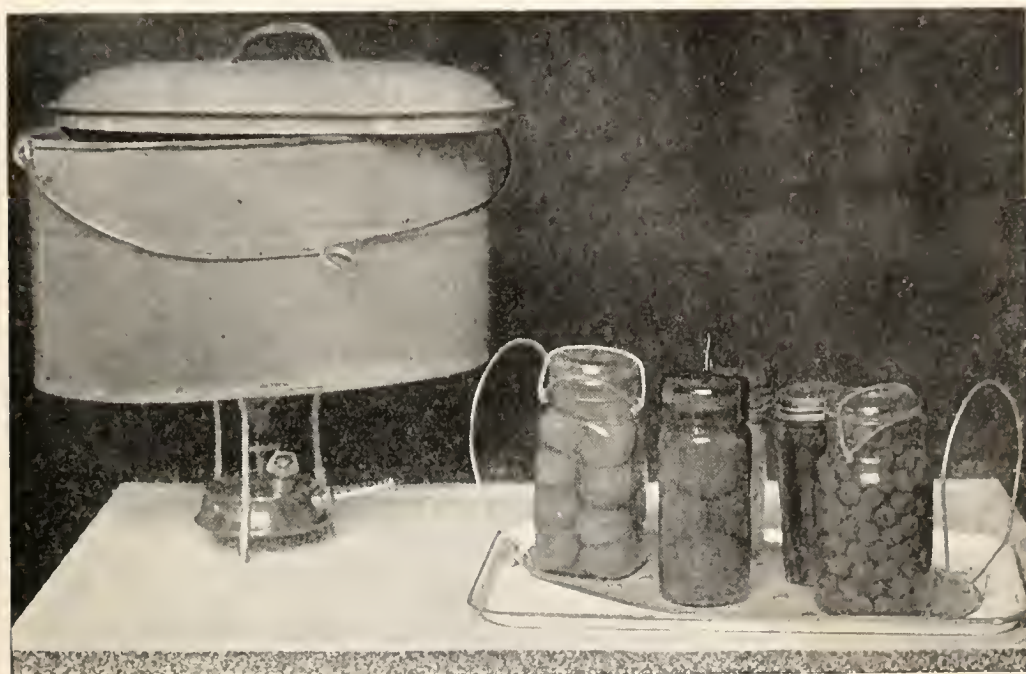
FIG. 19.—The processor and rack with jars ready to be sterilized. Note all clamps are raised and screw-top only partly screwed on.
