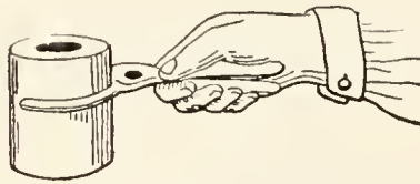
FIG. 20.—Tongs for handling hot cans.
