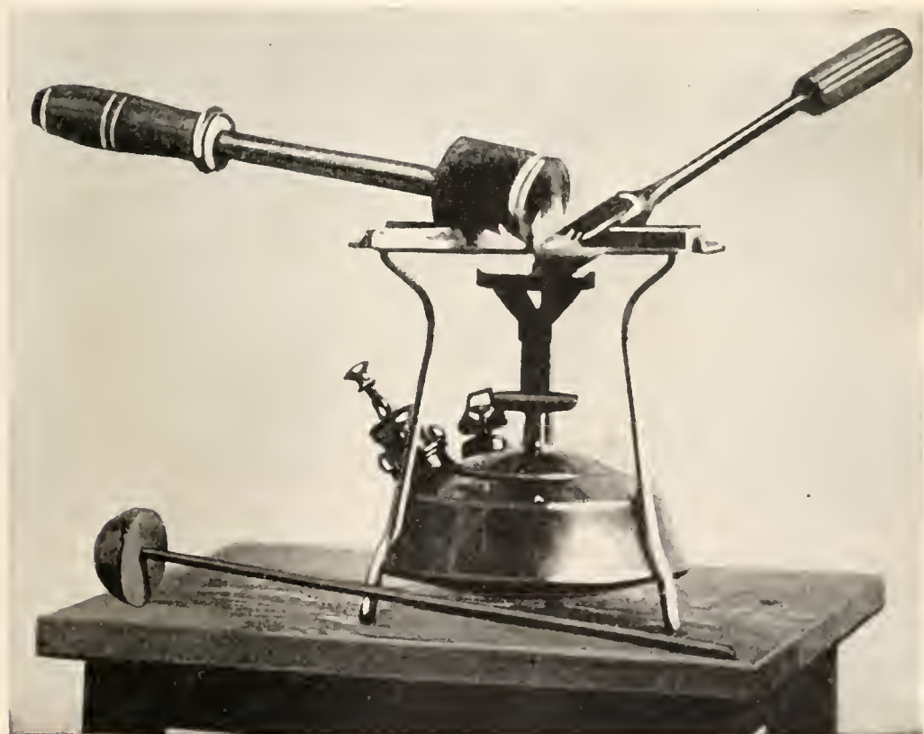
FIG. 28.—A kerosene stove which burns a gas flame for heating soldering tools.
