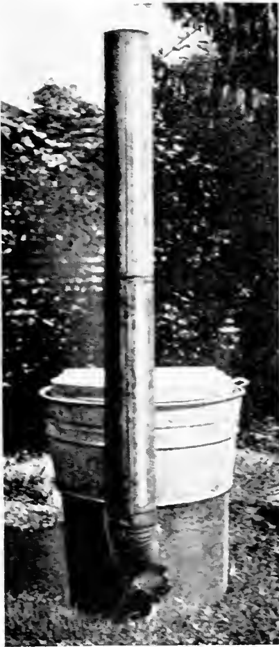
FIG. 56.—A homemade canner with brick fire-box and tub.
