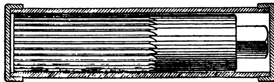
FIG. 10. BRASS-TUBE PROTECTION CASE FOR EXPENSIVE HAND REAMER
