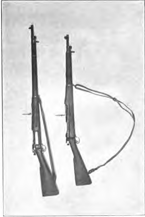
FIGURE 1.—U. S. Magazine Rifle, Model 1898 (Krag), Upper. U. S. Magazine Rifle, Model 1903, with Gun-Sling Adjusted for Firing, Lower.
