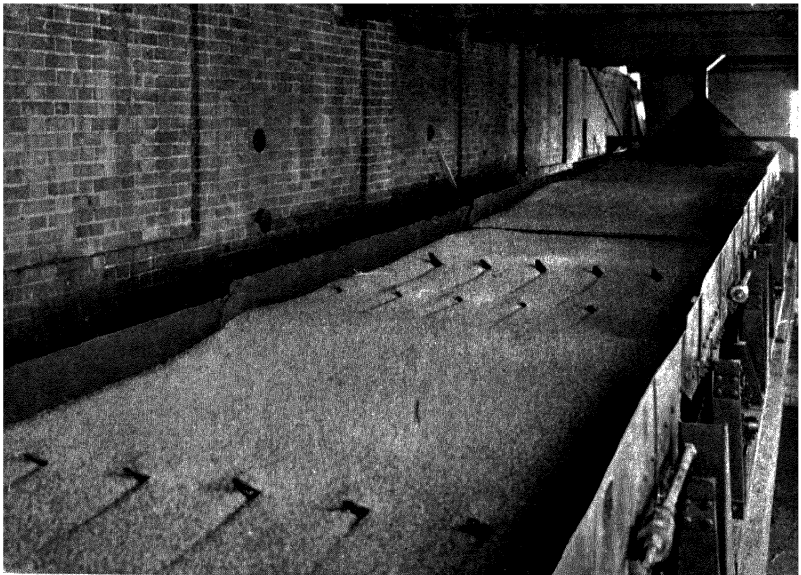
16 (b). Four Stage Butterley Goodall Dryer showing shaker buffers at side and weirs and ploughs
