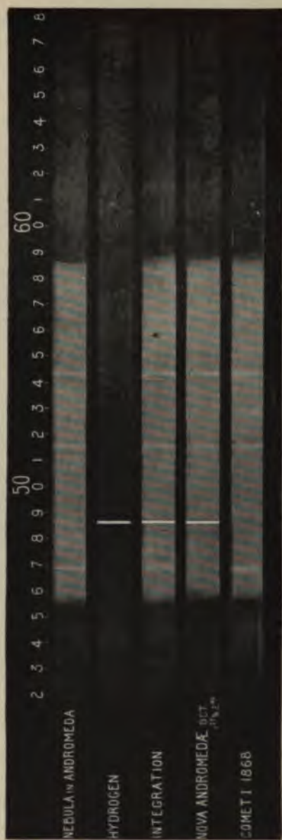
FIG. 40.—Spectra of the nebulae in Andromeda, Nova Andromedæ, and comet compared. The flutings common to all are those of carbon.
