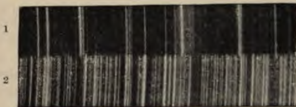
FIG. 33.—A small part of the Line spectra of barium and iron. 1, Barium. 2, Iron.
