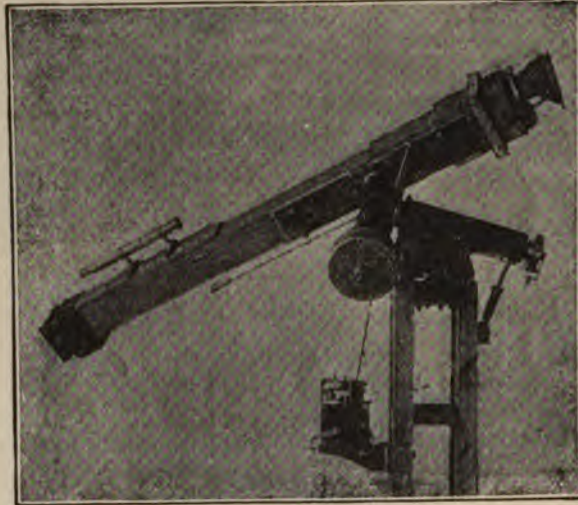
FIG. 6.—Showing method of photographing stellar spectra by the objective prism.
