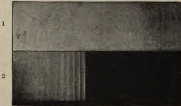
FIG. 35.—Spectra of burning magnesium compared with solar spectrum. (1) Sun. (2) Magnesium.
