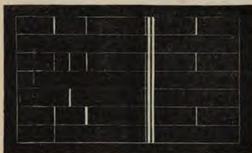
FIG. 72.—Showing the various intensities of the lines of magnesium as seen under different conditions.
