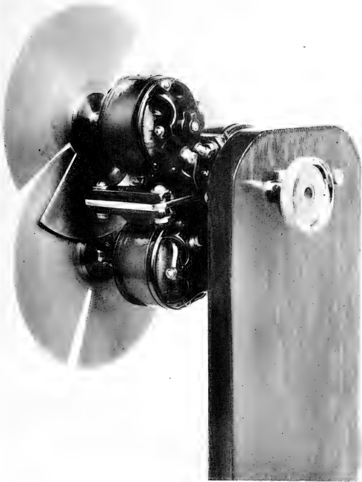
Electrically driven rotating sectors which graduate the intensity of the sunbeam to suit our instruments
