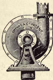
FIG. 21.—Centrifugal Pump. A, rising main ; B, suction pipe.
