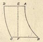
then when E F bisects A B C D,  $\frac{3 \text{ H}}{5} \text{ E A} + \frac{2 \text{ H}}{5} \text{ B F} = \frac{2 \text{ H}}{5} \text{ C F} + \frac{3 \text{ H}}{5} \text{ E D},$ 2 B F = 2 C F + 3 E D - 3 E A; for stability,
