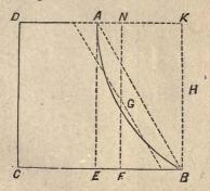
walls with a batter of that curve are also given, as they may be found useful in some cases. Let A G B in this figure be a curve
