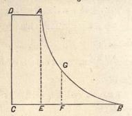
Moment of A B C D = (H × C E)  $\left(B E + \frac{C E}{2}\right) + \left(H \times \frac{2}{5} B E\right) (.734 B E) = (H × C E)$   $\left(\frac{5}{2} C E + \frac{C E}{2}\right) + (H × C E) \left(.734 \times \frac{5}{2} C E\right)$ = (H × C E) 3 C E + (H × C E) 1.835 C E = 4.835 H × C E<sup>2</sup>. Then 120 × 20 × 4.835 C E<sup>2</sup> = 160,000, C E = 3.71, B E =  $\frac{5}{2}$  3.71 = 9.28, and weight of wall
