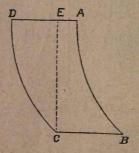
To find the moment of ABCD when the curves of the front and back of the walk are of different radii. Area of
