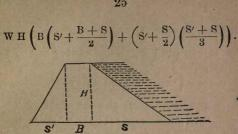
If in these last five equations W = 120lbs. to the cubic foot, H = 20 feet, S = 20feet, S' = 10 feet, and B = 10 feet, then the moment of the first section
