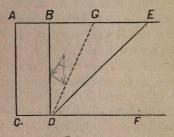
then if we bisect the  $\angle$  B D E by the line D G, B D G is the portion of the embankment supported by the retaining wall.
