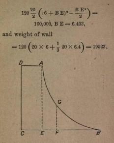
To find the moment of A B C D when A B E = A E C D. Then B E = 3 C E, area of A B E = H  $\times \frac{B E}{3}$  = H  $\times$  C E. Moment of
