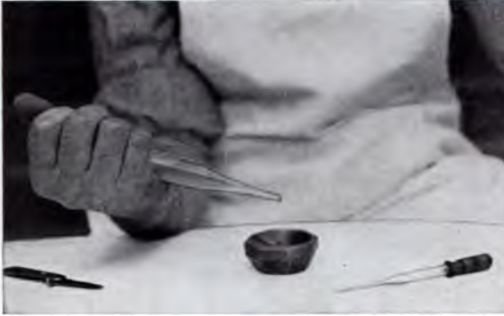
FIG. 242.—EXPRESSING A FEW DROPS OF EMULSION FOR STANDARDIZATION; HEAT OF HAND EXPANDS THE AIR IN THE TUBE, AND FORCES OUT THE FLUID.
