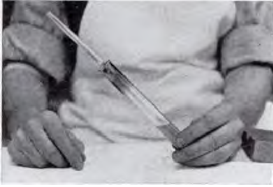
FIG. 237.—TUBE CONTAINING BACTERIAL EMULSION, WITH HANDLE ATTACHED AS AN AID IN SEALING.
