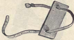
Fig. 106.—Pad for holding a staff and tripod.
