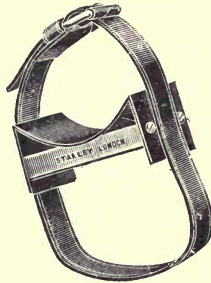
Fig. 107.— Improved pad for staff and tripod.
