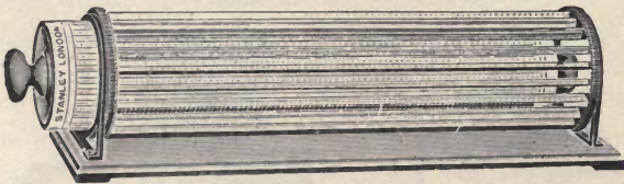
Fig. 430.—Thacher's slide rule.
