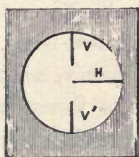
Fig. 75.—Stanley's platino-iridium point level stop.
