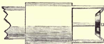
Fig. 221.— Conical reflector to illuminate axis of telescope.
