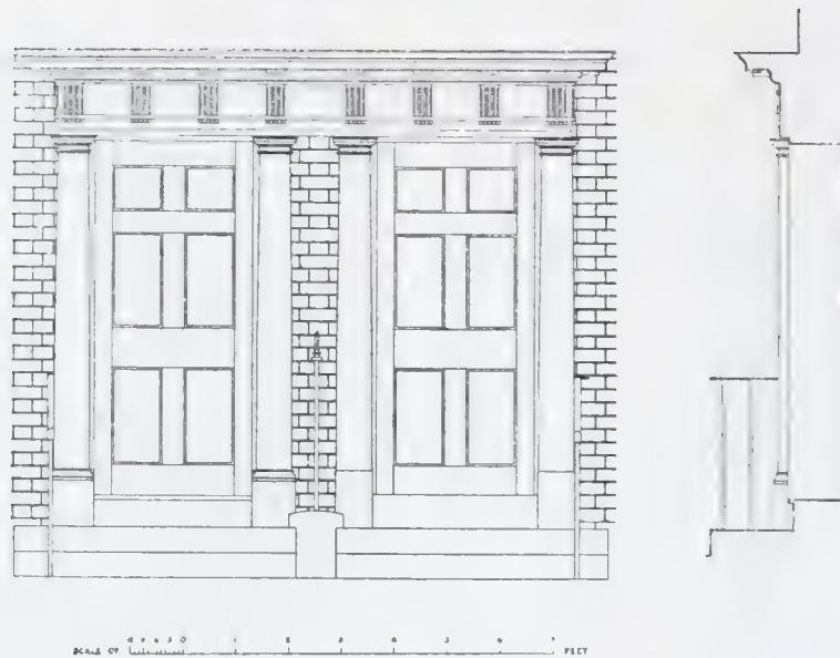
Fig. 17. Nos. 75 and 77 Kennington Lane, paired doorcases
