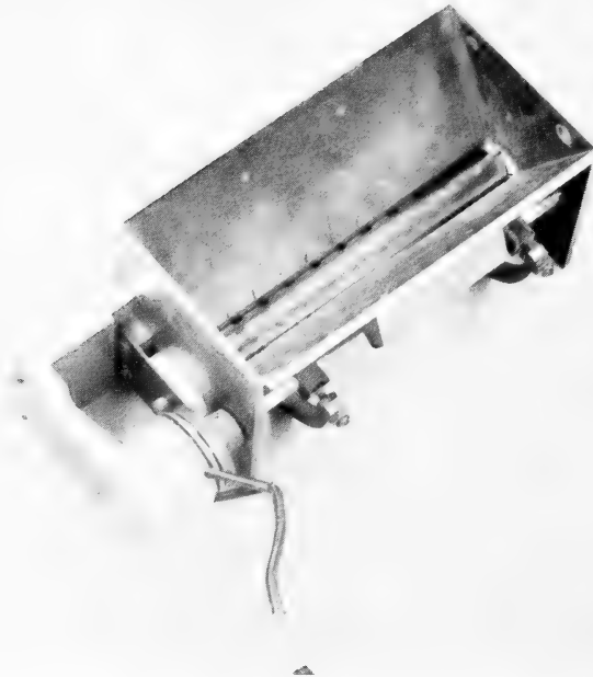
Fig. 1 Sand hopper. Sand is agitated by notched stirrer and falls through No. 60 drill holes at bottom of hopper. Delivery of sand is started and stopped by solenoid-operated valve on bottom of hopper.
