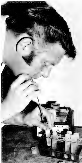
Figure 5. Serial dilution of samples for bacterial counts.
