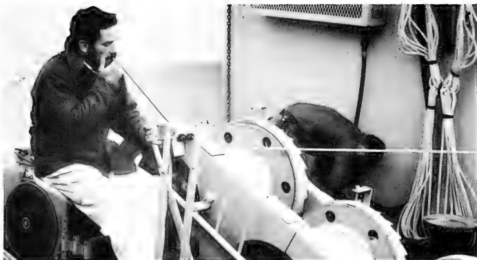
Figure 4. Winch for lifting and dropping sample line and anchor in the ocean.
