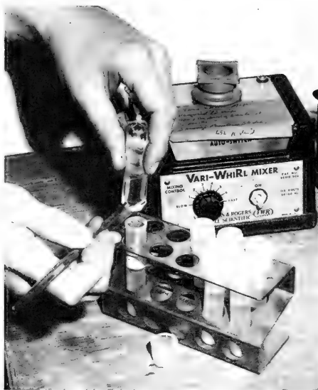
Figure 9. Emptying dialyzer bag into sterile test tube.
