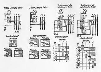
Fig. 4.—Ammeter switch connections.
