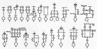
Fig. 169.—Typical connections of generators and bus.
