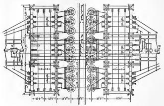
Fig. 268.—Plan view 110 K.V. outdoor station.
