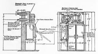
Fig. 90.—Westinghouse oil circuit breaker type CO1.
