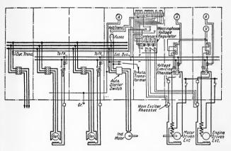
Fig. 219.—Typical connection exciter and field connections.
