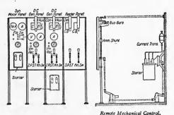
Fig. 187.—Arrangement of M.G. panels for mine service.
