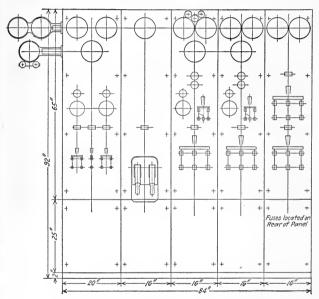
Fig. 221.—Typical low voltage Westinghouse switchboard.
