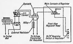
Fig. 161.—Excess voltage protection for regulator.
