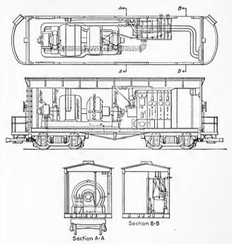
Fig. 255,-Portable substation for motor generator.
