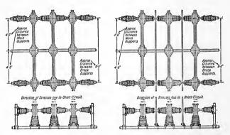
Fig. 237.—Heavy duty bus support.
