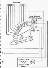
Fig. 164.—D.C. starter with low voltage release.
