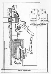
Fig. 37.—Cutter circuit breaker—solenoid operated.
