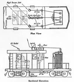
Fig. 212.—Sectional view of portable substation.
