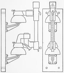
Fig. 23.—Disconnecting switch type of expulsion fuse.
