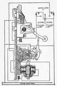
Fig. 36.—Cutter circuit breaker—motor operated.
