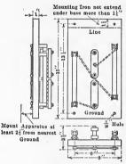
Fig. 133.-Non-arcing arrester.
