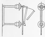
Fig. 26.—Fused circuit breaker.
