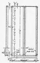
Fig. 178.—Angle framework for large switchboards.
