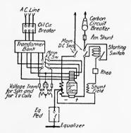
Fig. 202.—Diagram of D.C. starting of synchronous converters.
