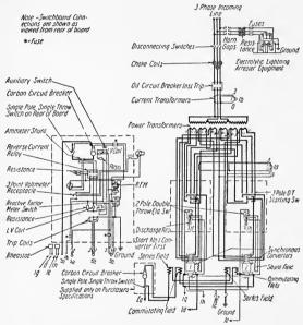
Fig. 205.—Diagram of connections for 1500-volt D.C. railway.
