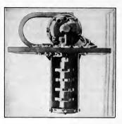
Fig. 210.—Westinghouse rotary drum switch for automatic substation.
