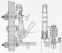
Fig. 46.—Westinghouse carbon circuit breaker, type CD.
