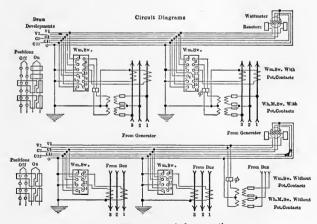
Fig. 5.-Wattmeter switch connections.
