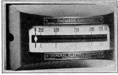
Fig. 108.—General Electric Co. horizontal edgewise meter.
