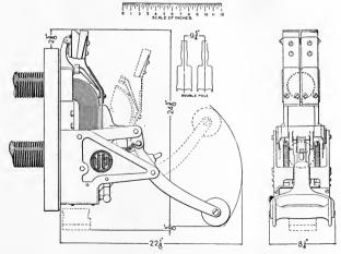
Fig. 34.—Cutter type LG carbon breaker.
