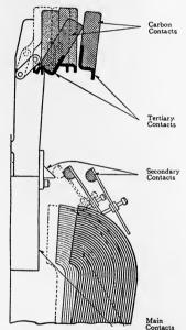
Fig. 49.—Westinghouse Type CA breaker—contact arrangement.
