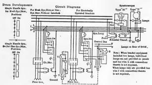
Fig. 7.—Connections for synchronizing to bus,
