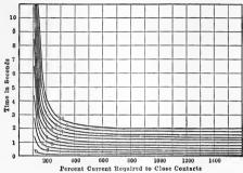
Fig. 100.—Relay characteristic curves.
