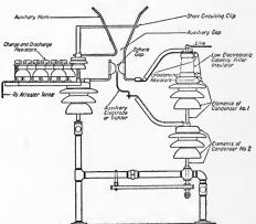
Fig. 137.—Westinghouse impulse gap for arrester.
