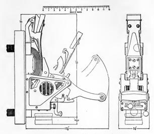
Fig. 33.—Cutter type LL carbon breaker.
