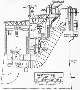
Fig. 263.—Sectional view Holter Plant, 110 K.V.
