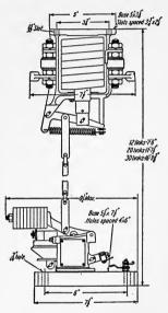
Fig. 106.—Series type of relay.
