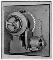
Fig. 155.—Motor operated field rheostat face plate.
