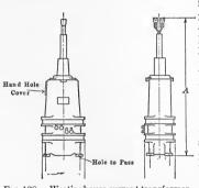
Fig. 128.—Westinghouse current transformer type "KC" double secondary.
