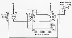
Fig. 165.—Automatic acceleration with series relay.
