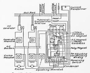
Fig. 157.—G. E. voltage regulator for A.C. machines.
