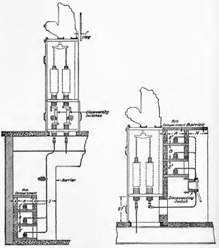
Fig. 248a.—Masonry compartments for motor operated breakers. (See Fig. 248b and c.)
