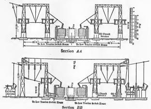
Fig. 269.—Section view 110 K.V. outdoor station.
