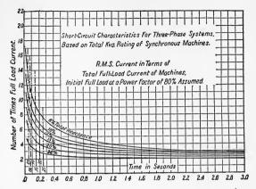
Fig. 53.—Short circuit characteristics—30 per cent. reactance or less.
