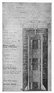
Fig. 135.—Section of electrolytic lightning arrester.
