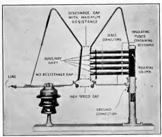
Fig. 142.—Schweitzer & Conrad graded resistance lightning arrester.
