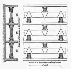
Fig. 236.—Bus bar supports with braces.
