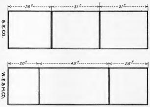
Fig. 181.—Three section panel.
