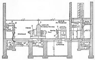
Fig. 253.—Sectional view of synchronous converter station.
