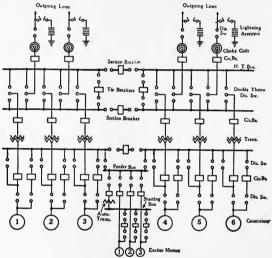
Fig. 174.—Diagram of connections for Rio de Janeiro.
