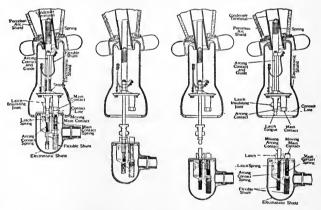
Fig. 93.—Westinghouse type GA oil circuit breaker—contact details.
