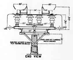
Fig. 17.—Horn-gap switch 70-K.V. double break.
