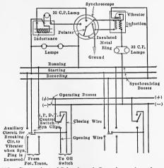
Fig. 110.—Connections of Schweitzer & Conrad record synchronoscope.
