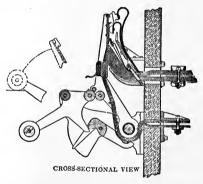
Fig. 45.—Roller-Smith carbon-break circuit breaker.
