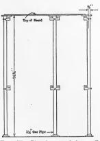
Fig. 177.—Pipe framework for small switchboards.
