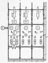
Fig. 204.—Switchboard for 1500-volt D.C. railway.
