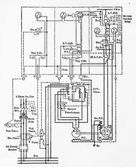
Fig. 188.—Diagram of connections for M.G. sets for mine service.
