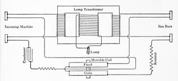
Fig. 123.—Diagram of connections. Weston synchronoscope.
