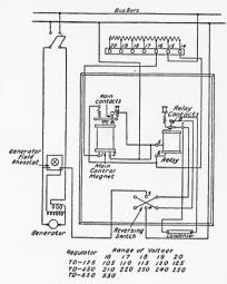
Fig. 156.—G. E. voltage regulator for D.C. machines.
