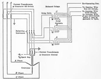
Fig. 105.—Schweitzer & Conrad multi-circuit relay.
