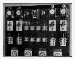
Fig. 175.—Wooden switchboard for Korea built 1887.
