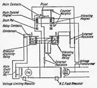
Fig. 159.—Westinghouse voltage regulator diagram.
