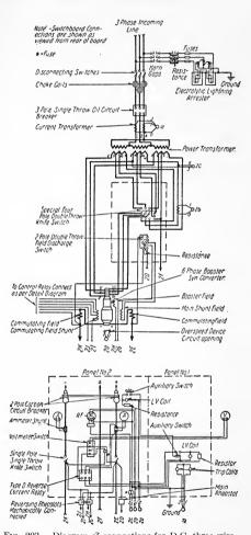
Fig. 203.—Diagram of connections for D.C. three-wire.
