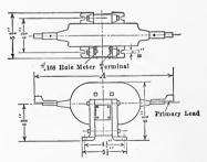
Fig. 127.—Westinghouse current transformer type "KA."
