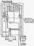
Fig. 186.—Connections of generator and battery panel.
