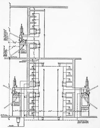
Fig. 250.—Masonry compartments for 22000 volts.
