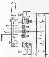
Fig. 2.- Motor starting knife switch.
