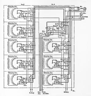
Fig. 184.—Diagram of connections with magnetically operated switches.
