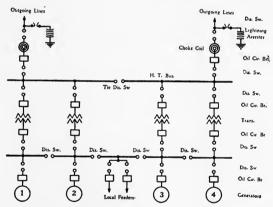
Fig. 173.—Diagram of typical plant with sectioned bus.
