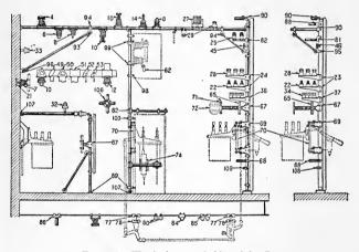
Fig. 239.—Westinghouse switchboard details.
