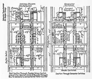
Fig. 251.—Section of switching galleries.
