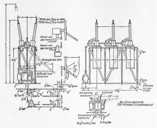
Fig. 91,-Westinghouse 37-K.V. oil circuit breaker type G11.
