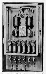
Fig. 158.—Westinghouse automatic generator voltage regulator.
