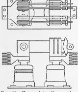
Fig. 11.—Heavy duty disconnecting switch.
