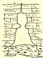
Fig. 67.—Section of a mine in this ore deposit (shown in Fig. 66) after it is worked out. (Chamberlin.)
