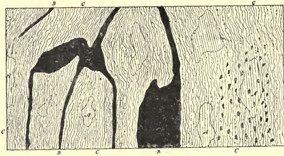
Fig. 53.—Section exposed in a pit at the Dobbins mine in Georgia. The black bands represent manganese ore, and the shaded portion clays. (Penrose.)
