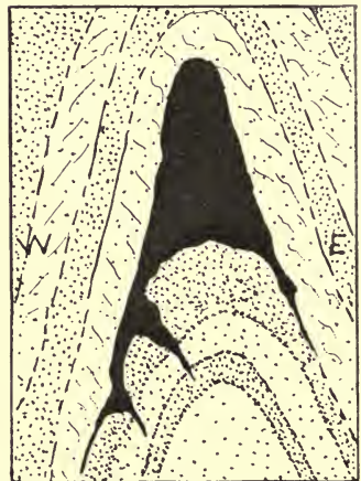
Fig. 90.—Section of a "saddle reef," or lode, New Chum Consolidated mine, Bendigo gold field, Victoria, Australia. (Schmeisser.)
