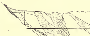
Fig. 80.—East-west section through the Comstock lode in Nevada, showing the position of two of the ore-bodies, and of the Suro tunnel.
