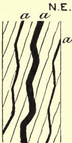
Fig. 95.—Section in the Victor, Smuggler Lee, and Buena Vista mines, Cripple Creek district, showing the parallel ore-bodies ( a ). (Penrose.)
