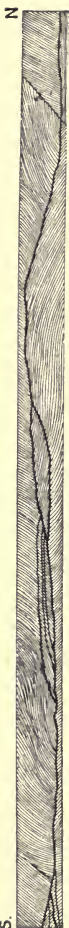
Fig. 22.—Horizontal plan in the C. O. D. Mine, Cripple Creek, Colorado, showing system of fissures. (Penrose.)
