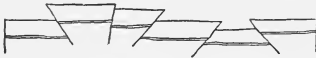
Fig. 19.—Reversed faults in horizontal rocks that have broken the original beds but left them parallel.
