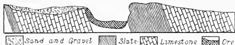
Fig. 38.—Section showing the geology of the Cambro-Silurian iron ore deposit of the Amenia mine, Dutchess county, N. Y. (Putman.)
