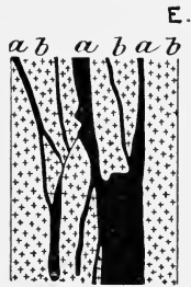
Fig. 97.—Section showing the forms of the vein in the Blue Bird mine, Cripple Creek district. The ore is shown black, b is the country rock. (Penrose.)
