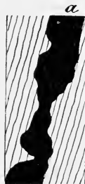
Fig. 96.—Another section showing the form of the ore-body in the Victor, Smuggler Lee, and Buena Vista mines, Cripple Creek district, Colorado. (Penrose.)
