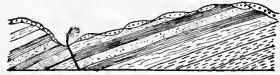
Fig. 138.—Section to illustrate the geologic reason for a spring upon a fault line.
