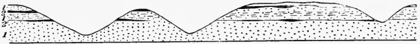
Fig. 11.—Geological section in the manganese region of North Arkansas. The black bands represent beds of manganese that were deposited in layers alternating with the accompanying rocks.
