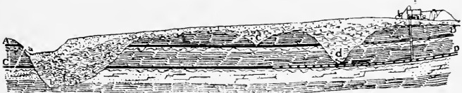
Fig. 116.—Geologic section in the glaciated part of the coal region of Indiana, showing how the outcrops are mostly concealed by drift. (Ashley.)
