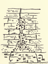
Fig. 66.—Section showing the zinc ore deposit in the Atkinson range in Wisconsin. (Chamberlin.)
