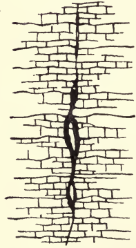
Fig. 18.—Gash vein in magnesian limestone of Wisconsin. (Chamberlain.)
