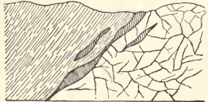
Fig. 31-32.—Examples of contact deposits or ore-bodies at the contact between two different kinds of rock.
