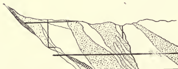
Fig. 80.— East-west section through the Comstock lode in Nevada, showing the position of two of the ore-bodies, and of the Sutro tunnel.
