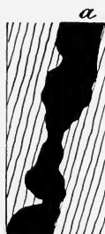
Fig. 96.—Another section showing the form of the ore-body in the Victor, Smuggler Lee, and Buena Vista mines, Cripple Creek district, Colorado. (Penrose.)
