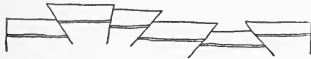
Fig. 19.—Reversed faults in horizontal rocks that have broken the original beds but left them parallel.
