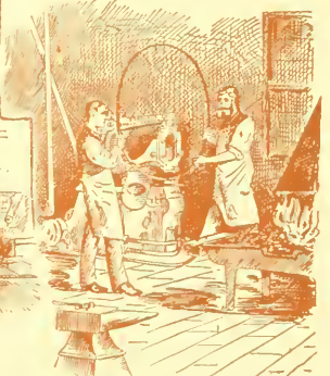
"THE FORGE" WELDING A TIRE WITH THE HELVE HAMMER
