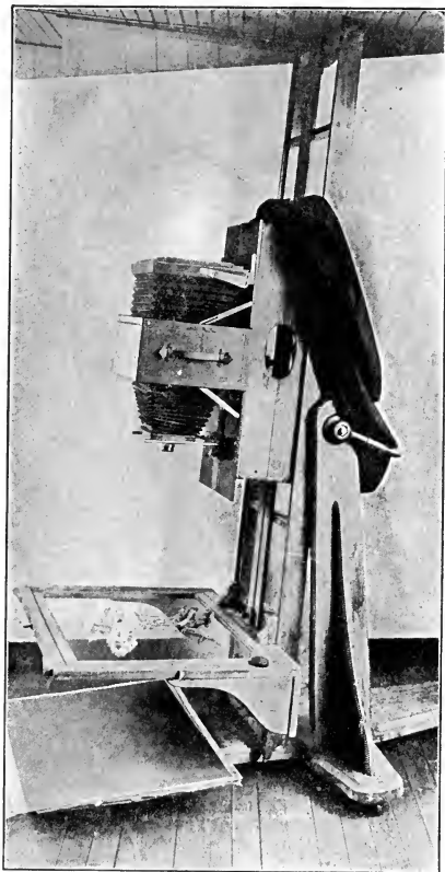
FIG. 6—APPARATUS FOR VERTICAL PHOTOGRAPHY (McFARLAND)
