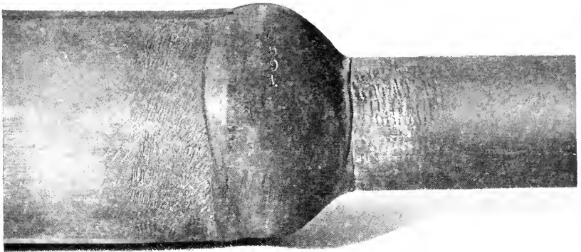
Fig. 1—A conventionally wiped joint between telephone cable and sleeve (third size).
