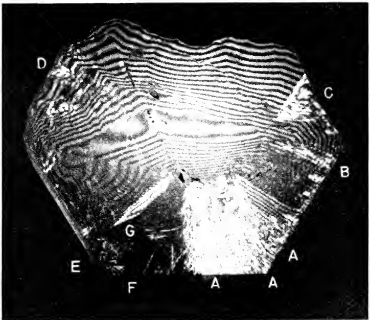
Fig. 4.9—The same cap as in Figure 4.8, but viewed slightly off the optic axis. Note the increased number of thickness-contours, and their fineness, also that some twinning regions are enhanced.
