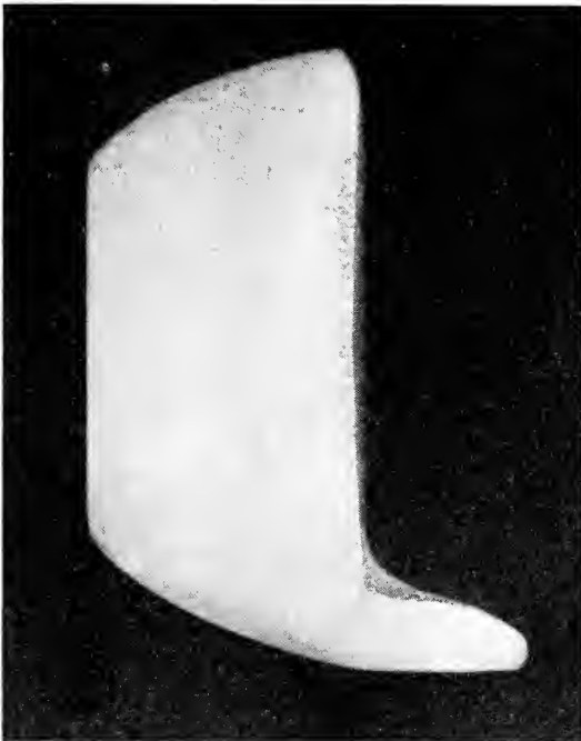
Fig. 5—An ingot of wiping solder which had been tilted while in the crucible before completely solidified. The lower lip represents eutectic drainage from the partially solidified mass (magnification 1\frac{1}{2} \times ).
