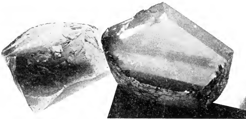
Fig. 4.1—Quartz may show smoky or citrine coloring throughout or only in restricted regions, irregularly as at the left, or in PHANTOM planes as at the right.
