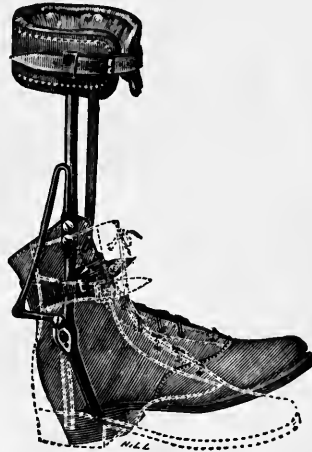
Fig. 497.—Ernst's Apparatus with Toe-elevating Spring for Paralysis of lower Extremity below the Knee Joint. The dotted line shows the position of the boot when the action of the spring is overcome by the weight of the body. The figure indicates the action of the spring.
