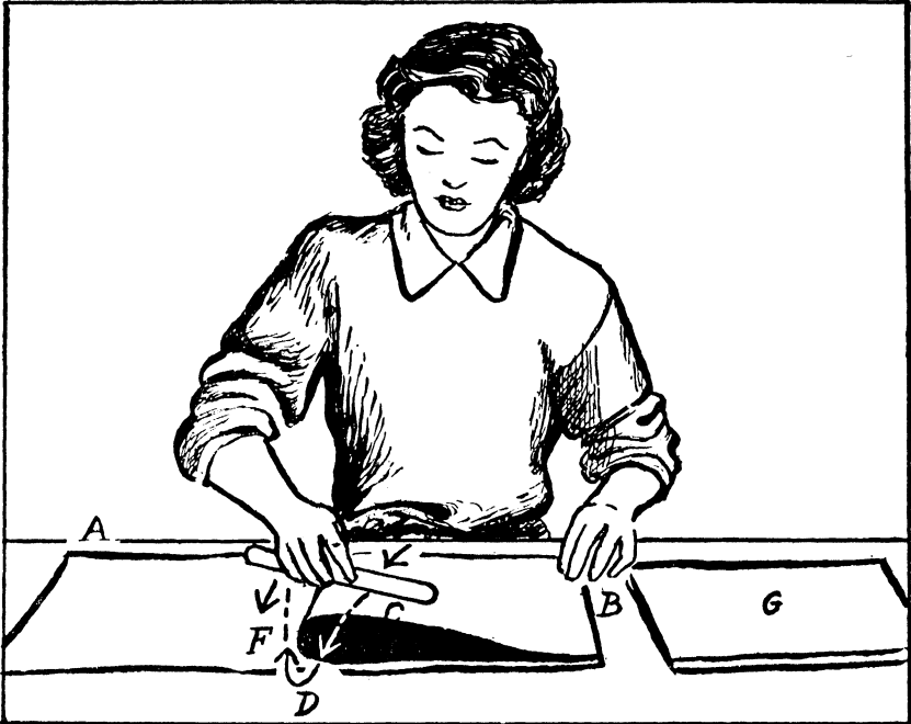
Figure 50. Path of hand in creasing folded sheet of paper—old method. Two fold. In Figure 51, the improved method, a smooth “S” curve made by the by permission from Motion and Time Study —3rd Ed., by R. M. Barnes,
