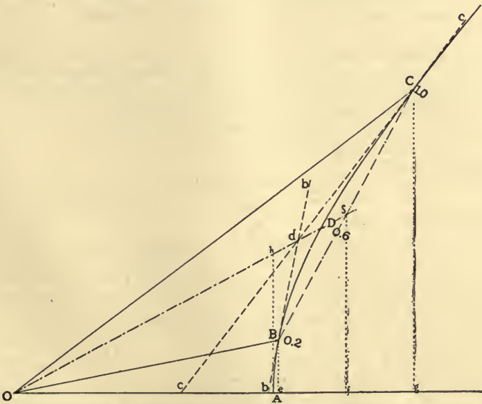
FIG. 18. — Bisection of a hyperbolic sector by a radius vector through the intersection of terminal tangents, or through the midpoint of the chord between terminal points.
