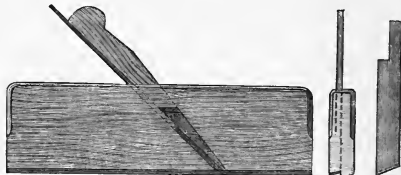
Fig. 64. Dove-tail Filletster, seen from the side and from behind. \frac{1}{2} .
