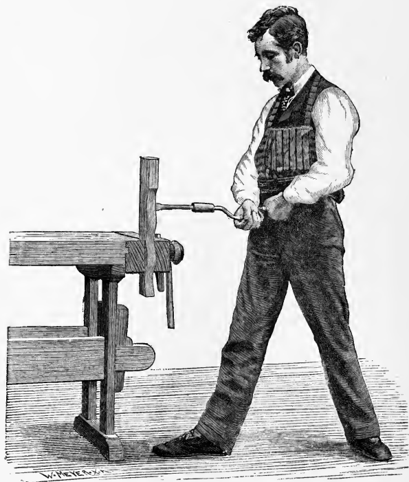
Plate V. Position: Horizontal boring with the brace.
