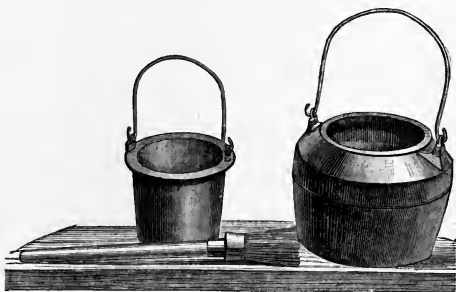
Fig. 86. Glue Pot (inside pan) and Brush.
