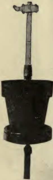
FIG. 24. — Gauge for measuring root pressure. \times \frac{1}{2} .
