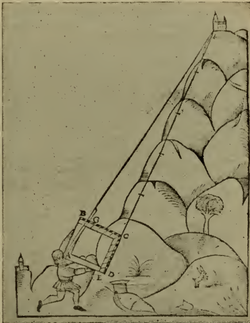
THE QUADRANT USED FOR ALTITUDES Finæus's "De re et praxi geometrica," Paris, 1556
