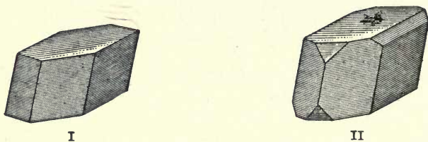
Fig. 9. Typical Monolinic Crystals of Sucrose, I. Tabular Form, II. Form with Hemihedral Faces. 20
