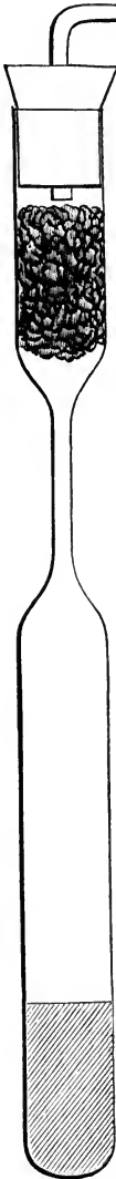
FIG. 45. — Gruber's tube for anaerobic cultures. Ready for use. Somewhat reduced in size. (After Gruber.)
