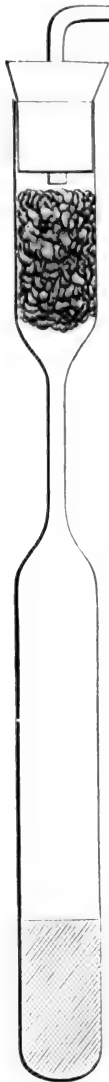
FIG. 45.—Gruber's tube for anaërobie cultures. Ready for use. Somewhat reduced in size. (After Gruber.)
