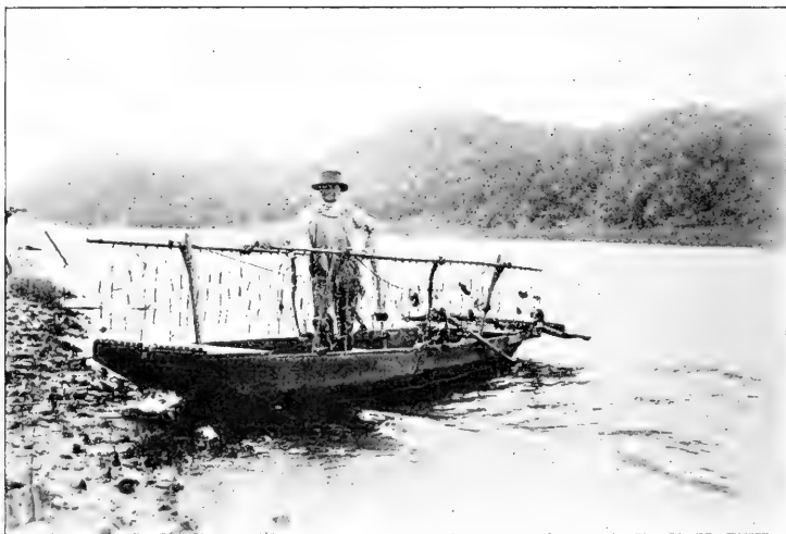
Fig. 49. A flat-bottomed dredging boat rigged with two crowfoot dredges, with typical fisherman, McGregor, Iowa. Note the shore strewn with dead shells. This is an example of the waste of raw material which has now largely ceased following the educational movement inaugurated by the U. S. Bureau of Fisheries through the biological station at Fairport, Iowa. Photograph by Frank M. Woodruff.
