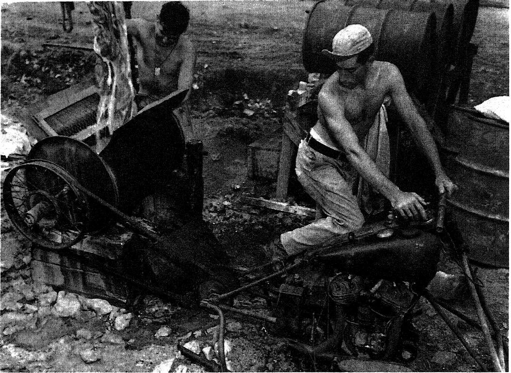
MAKESHIFT WASHING MACHINE built from a steel drum and a motorcycle, Port Moresby, New Guinea.
