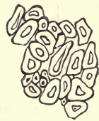
FIG. 27.— Cross-section of jute fibres.
