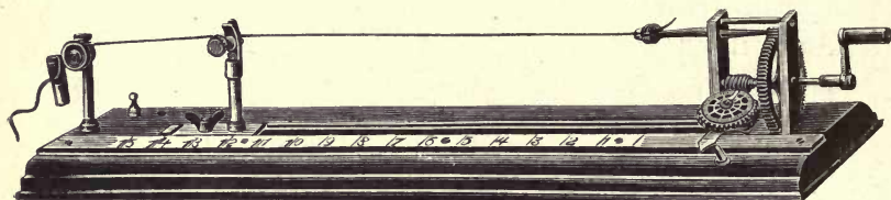
FIG. 49.—Heal's twist tester.
