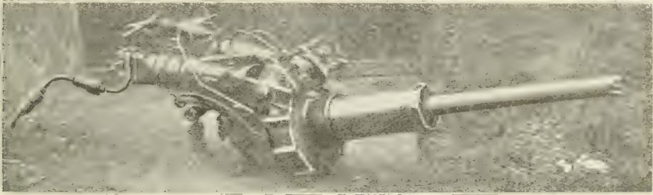
BRANDT HYDRAULIC PERFORATOR USED IN BORING SIMPLON TUNNEL. The cutting teeth at end of stem are cooled by running water forced through hollow shaft.
