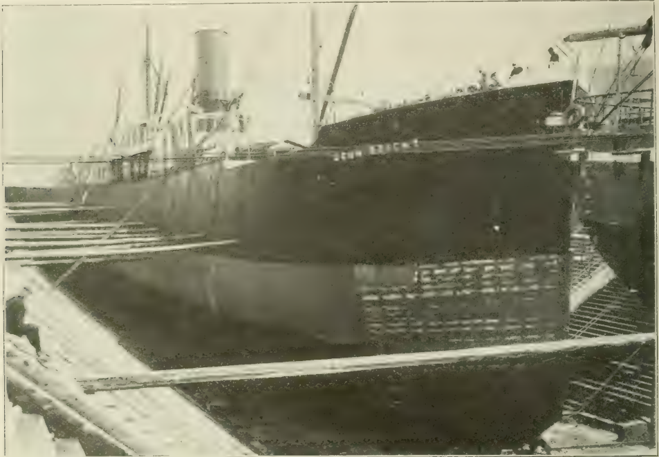
SS. JOHN BRIGHT TEMPORARILY FITTED WITH WOODEN BOW.
