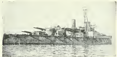
THE FIRST BRITISH BATTLESHIP WITH BUT ONE MAST—THE Hercules . Her armament consists of ten 12-inch guns with a full broadside. She has a displacement of over 20,000 tons.
