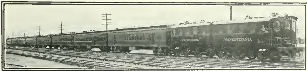
A PENNSYLVANIA ELECTRIC LOCOMOTIVE WITH TRAIN OF ALL-STEEL CARS FOR USE IN THE HUDSON RIVER TUNNEL.
