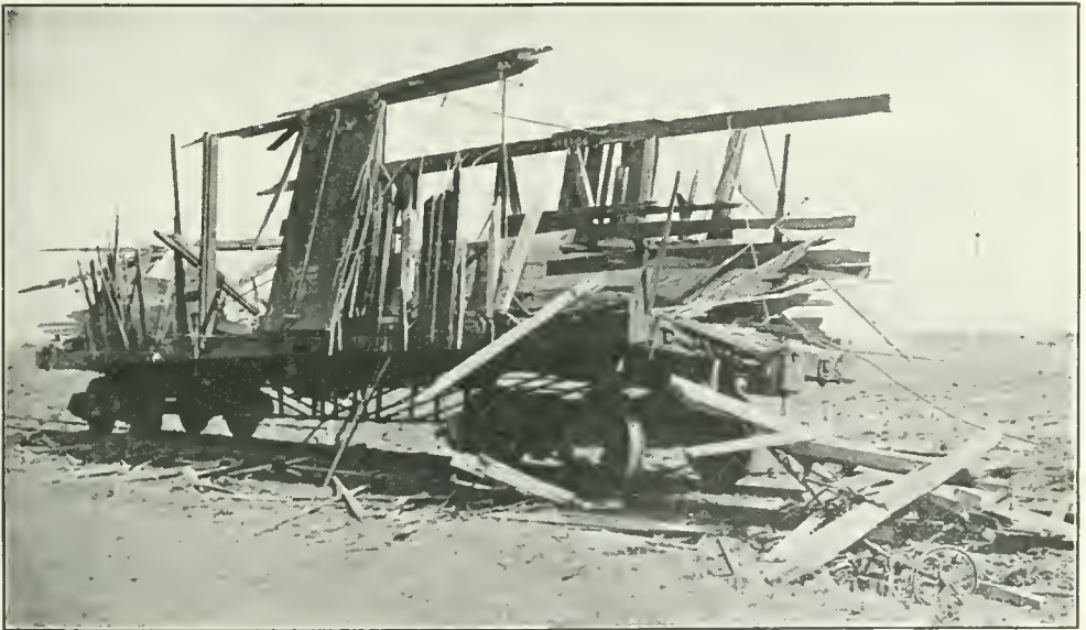
A HEAVY BOX CAR JARRED TO PIECES ONE-HALF MILE FROM THE EXPLOSION.
