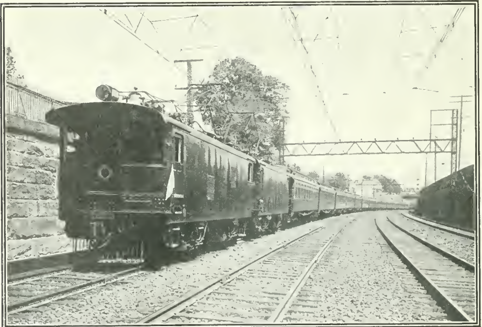
DOUBLE ELECTRIC LOCOMOTIVE TRAIN OF FOURTEEN PASSENGER COACHES. Single-phase electrification overhead is the triangular or older form of construction.
