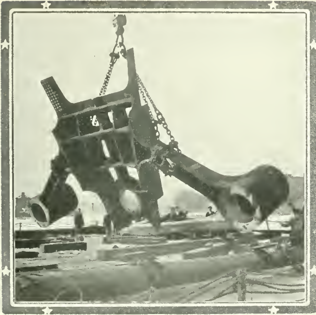
BRINGING THE "AFTER BOSS ARMS" INTO POSITION. One of the gigantic parts of the Olympic . Weight, 72½ tons.
