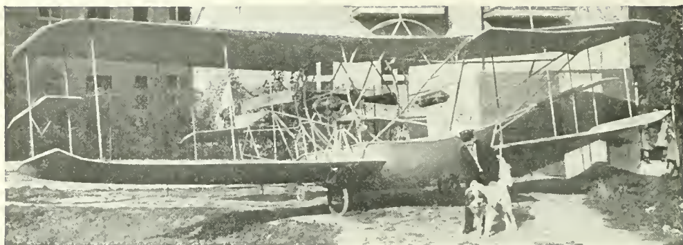
A FRENCH AEROPLANE THAT CAN FLY IN THE AIR AND RUN OVER LAND OR WATER. When traveling along the ground or through the water, the planes are detached.
