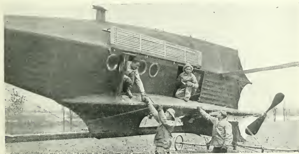
AFFORDS PROTECTION AGAINST WIND AND WEATHER. A pneumatic system aids the aviator in controlling the machine.
