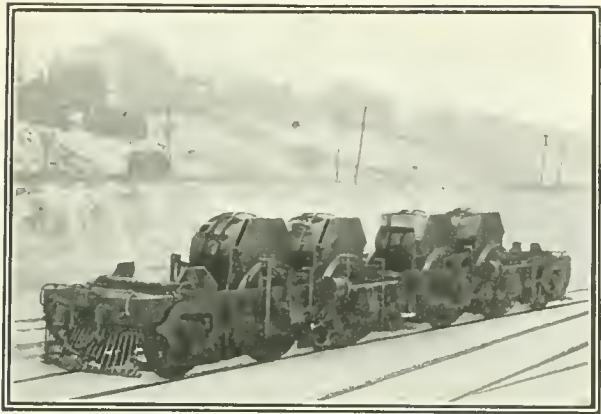
ARRANGEMENT OF MOTORS OVER DRIVING AXLES. For the single-phase and direct current locomotive—passenger and freight service—on the New York, New Haven and Hartford Railroad.
