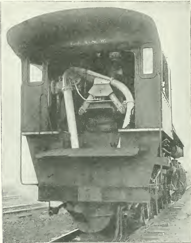
REAR VIEW OF LOCOMOTIVE WITH THE STREET STOKER.
