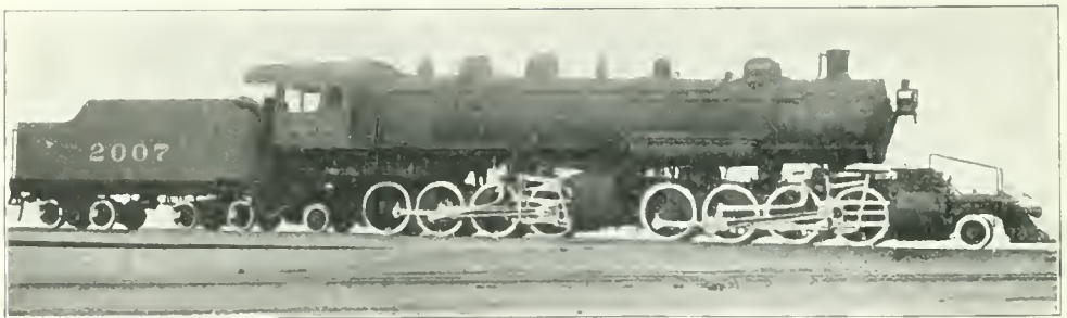
A MALLET COMPOUND LIKE THIS COULD BURN 12,000 TO 15,000 POUNDS OF COAL PER HOUR IF DESIRABLE OR NECESSARY There is no way, however of getting it into the fire-box.
