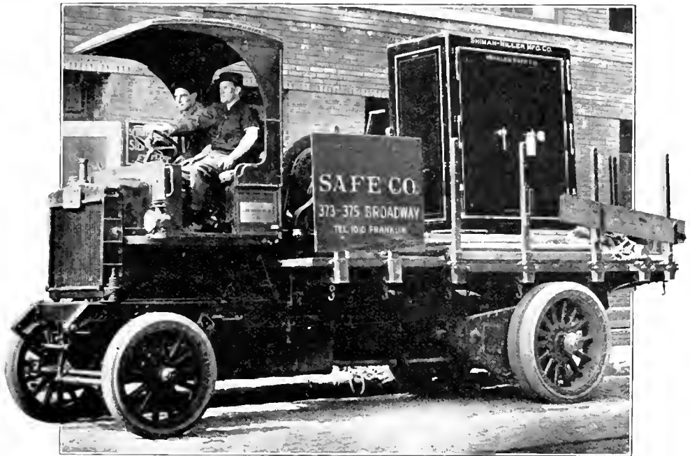
A MOTOR TRUCK EQUIPPED WITH WINDLASS FOR RAISING AND LOWERING SAFES.
