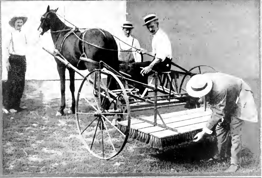
THE MACHINE FOR POLLENIZING CLOVER. Note the "fuzzy fingers" which the stooping man is touching.
