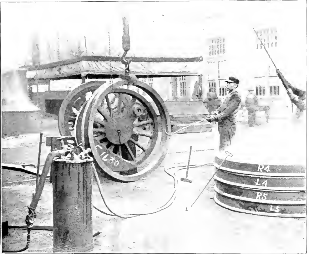
METHOD OF HEATING COMPLETE SET OF TIRES AT ONE TIME WITH CRUDE OIL BURNER. This is the new method. Formerly a piece of red hot gas pipe was placed around the tire to expand it. It was a slower process.
