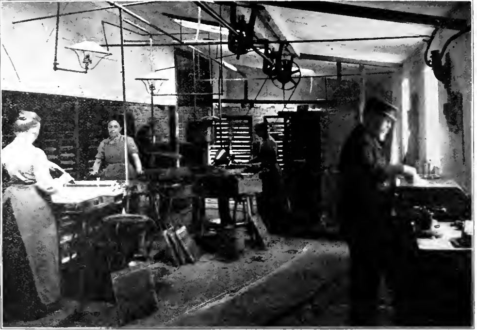
IMMERSING THE MATCHES IN THE IGNITING COMPOSITION. White phosphorus renders this occupation a deadly peril.
