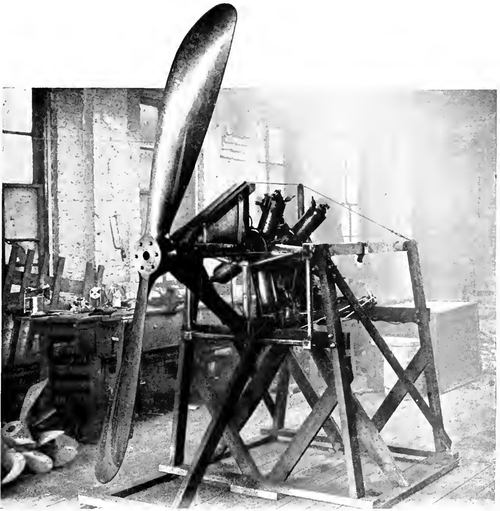
THE BROOKE MOTOR FITTED WITH A PROPELLER FOR DRIVING AN AEROPLANE.
