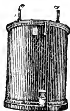
The First 10,000 Volt Transformer
