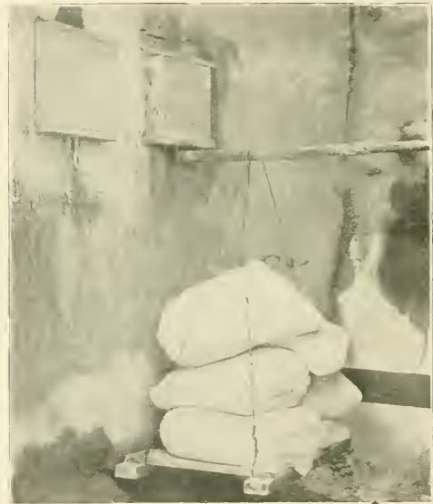
Fig. 7. Showing test to determine adhesion of gunite to asphalt membrane
