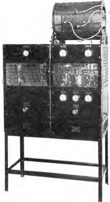
Figure 6—HIGH POWER TRANSMITTER FOR POWER LINE TELEPHONE COMMUNICATION.
