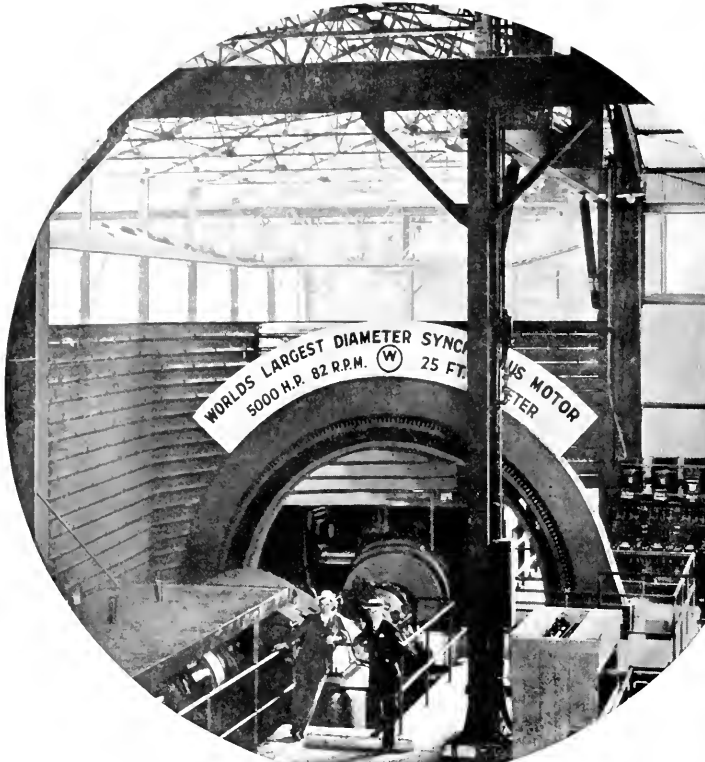
This 5000 h.p. motor in the Columbia Steel Company's Plant, with its frame of arc-welded steel, is physically the largest synchronous motor ever built.
