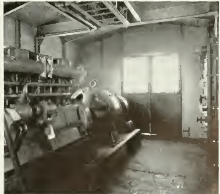
—Courtesy Westinghouse Electric & Mfg. Co. The 127-h. p. motor which drives the portable mooring mast for the Akron
