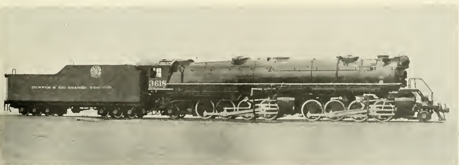
Railways are looking for more economical designs in locomotives in order to cut down operating expenses. This locomotive is one of the late types, built for the Denver and Rio Grande Western by the American Locomotive Company. It is of the four cylinder simple class, twelve-wheeled tender type.
