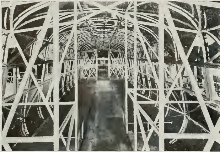
HERE'S HOW—the framework of the light weight, streamlined rail cars for high speed is Lindewelded from chrome-molybdenum steel tubing.
