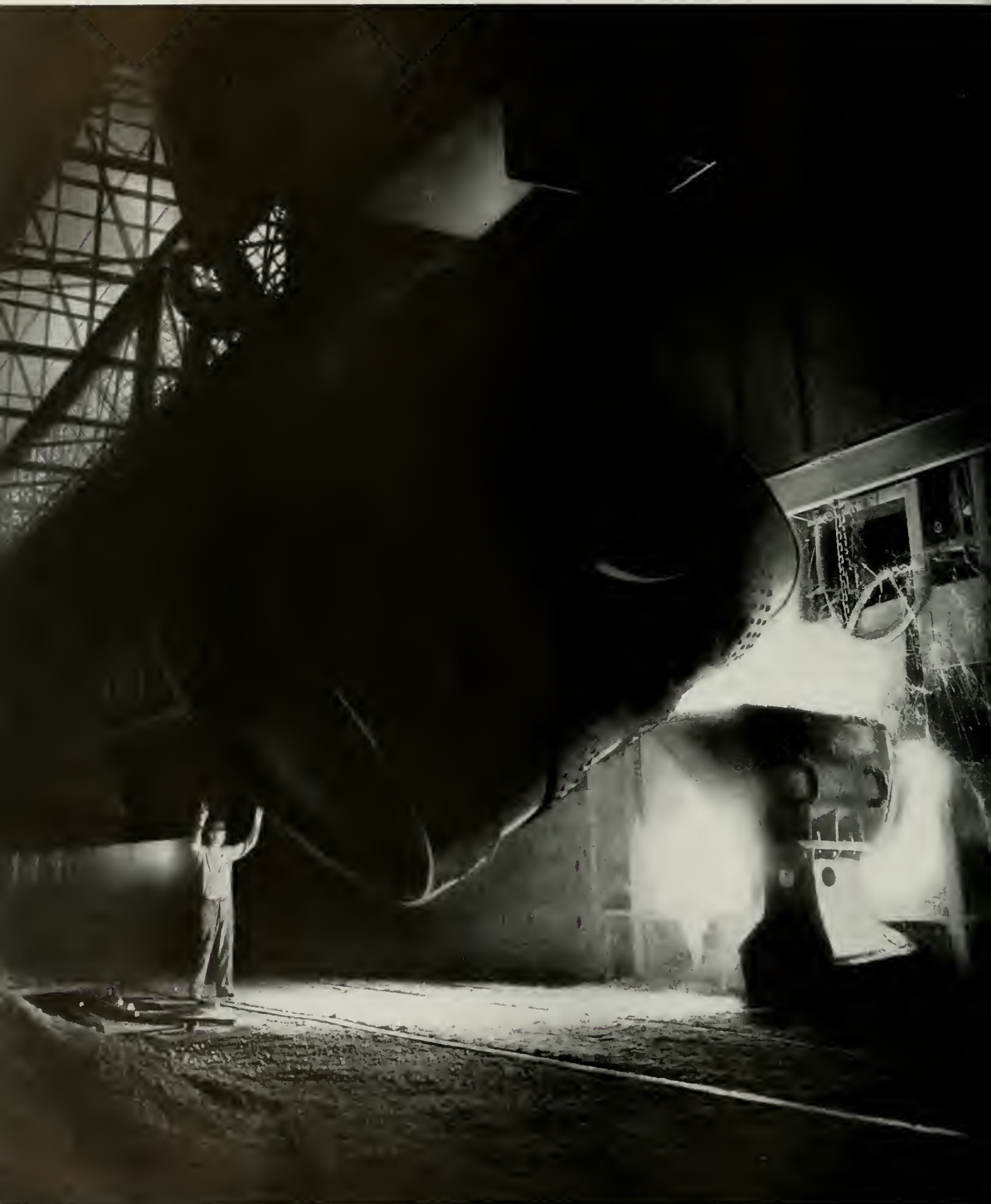
THERE WERE GIANTS IN OLDEN TIMES—AND THERE ARE TODAY At man's command 100 tons of liquid pig iron is being poured into the open-hearth furnace.
