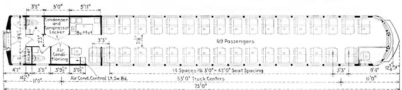
Floor plan of seventy-five-foot "Illini" indicates comfortable seats for sixty-nine passengers
