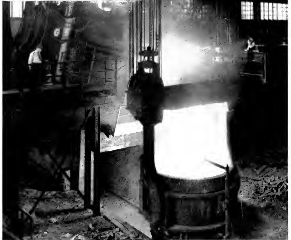
Pouring a heat of Timken Electric Furnace Alloy Steel at the Timken steel plant.
