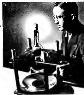
Dr. D. W. Epstein with a projection television tube, reflector and lens unit. Here the image on the end of the tube hits the reflector, is corrected by the lens, projected to the screen, then enlarged . . . making possible larger and clearer television than ever before.
